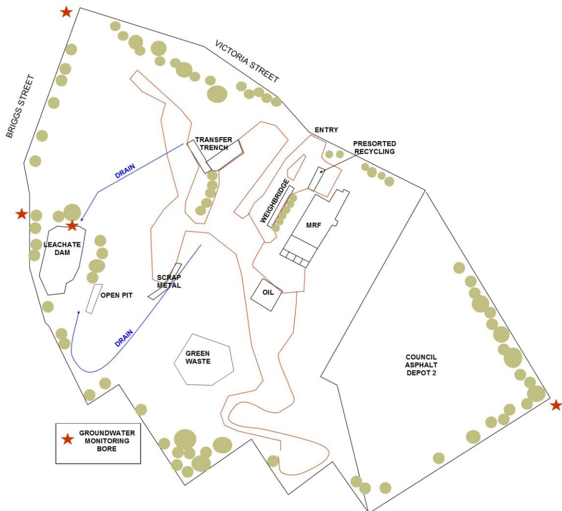
Image 2: Site Plan indicating drainage and leachate dam.
